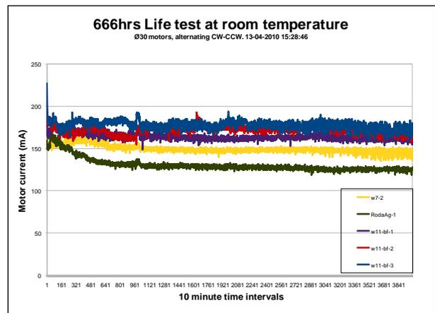
Figure 19 – Test of Ø30mm motors for continuous operation at room temperature
