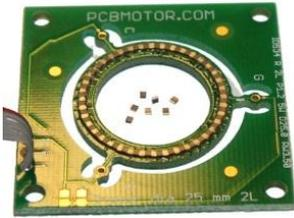
**Figure 6** – Stator with piezo components in center
