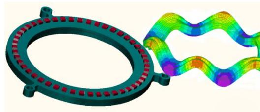
**Figure 3** – 30mm stator ring (left) and 6-wave stator model
