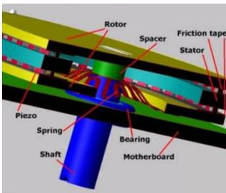
**Figure 10** – Cross section of motor construction
