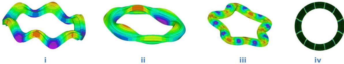
**Figure 4** - Traveling wave principle at different frequencies 1 to 3, 4<sup>th</sup> is sand pattern for good resonance frequency.
