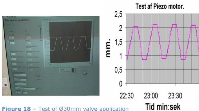
Figure 18 – Test of Ø30mm valve application +1000 Hrs. ~125,000 activation
