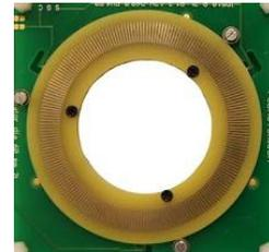
**Figure 13** – 40mm hollow center rotor.
