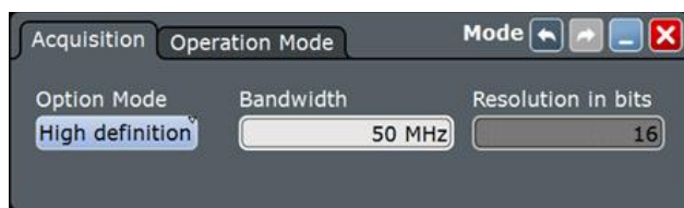
Abb. 4: Option R&S®RTO-/R&S®RTE-K17 – High-Definition-Mode
