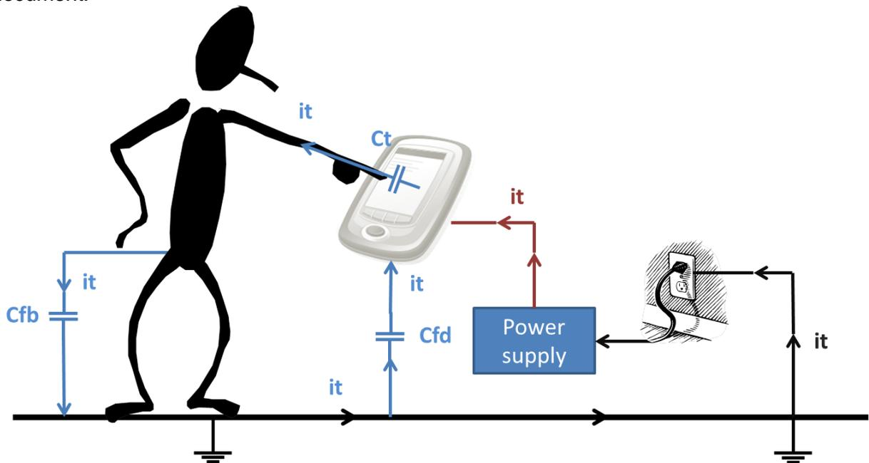
**Figure 4 - idealized model of a tethered device**
