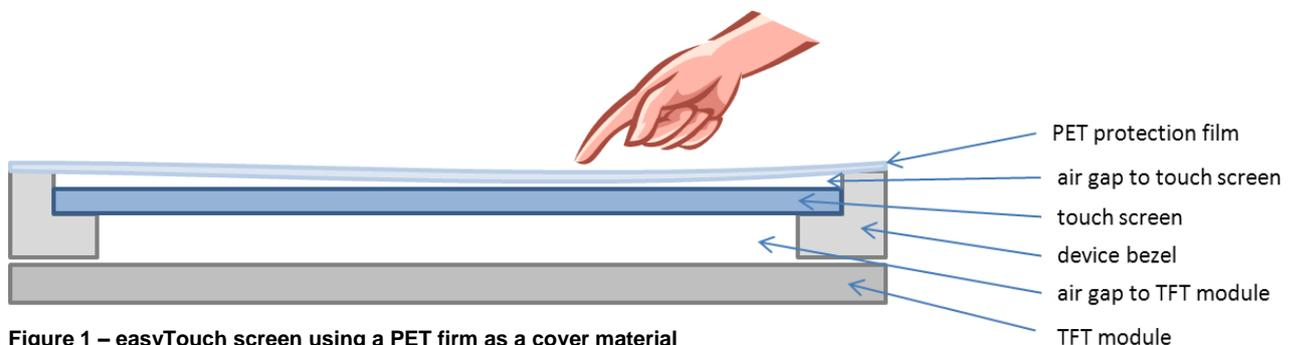
Figure 1 – easyTouch screen using a PET firm as a cover material
