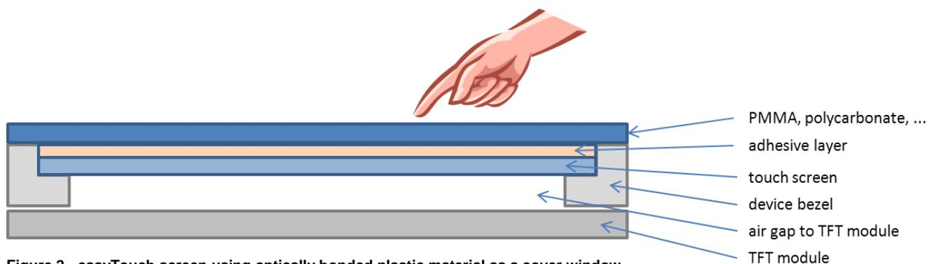
Figure 2 - easyTouch screen using optically bonded plastic material as a cover window
