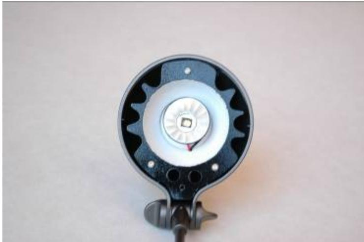
Figure 5a: Cree MC-E including reflector optic
