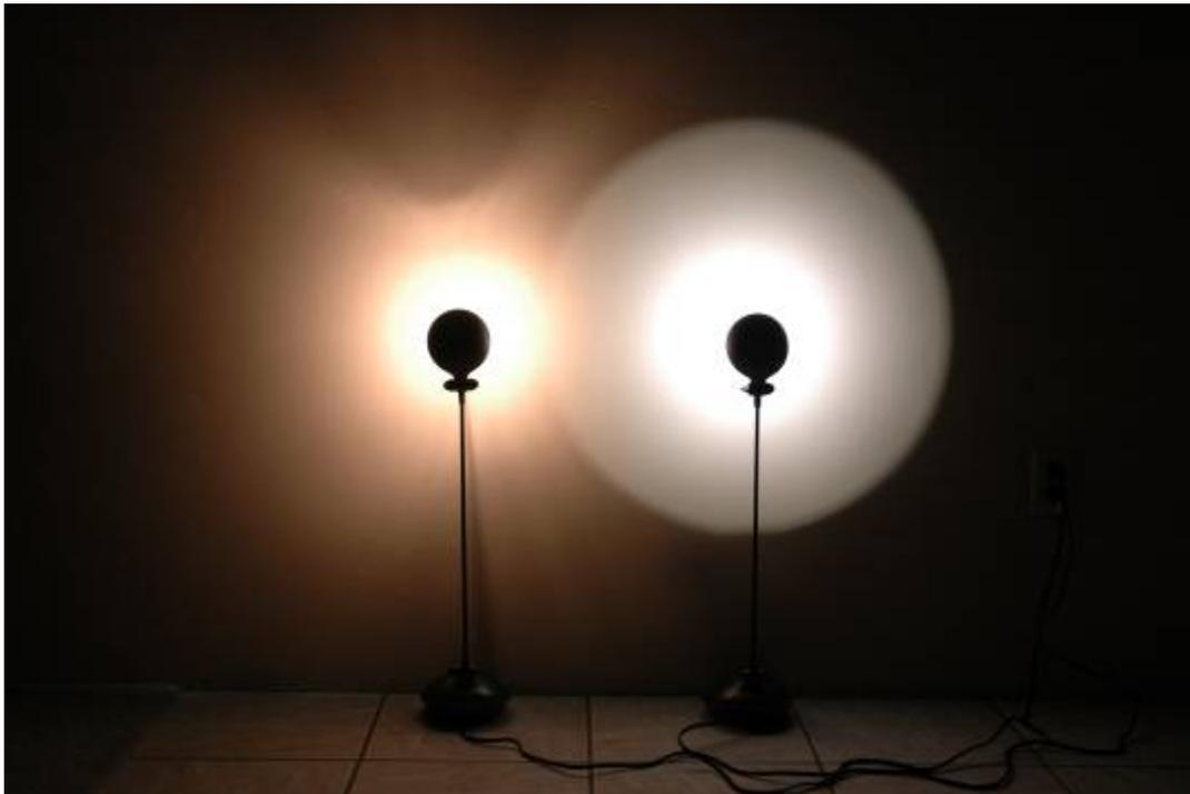
Figure 9: Light pattern of 35W Halogen and LED lamps
