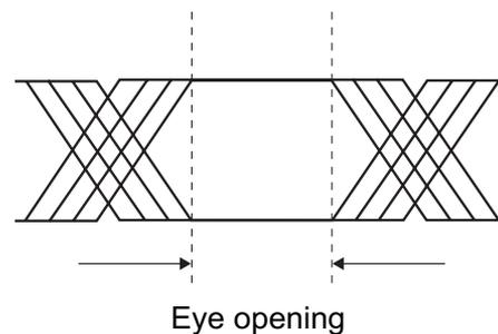
Jitter in the signal closes the “eye” and make data and clock recovery more difficult.
