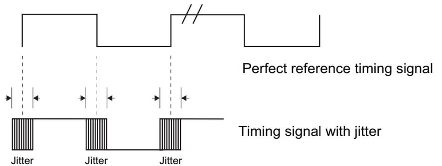
Note: Jitter around each edge can be different and may not be equally distributed around an edge. Also jitter in the next periods can be different.
