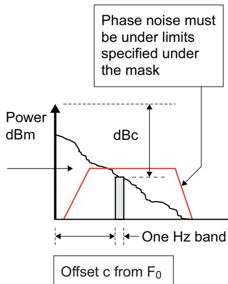
**Figure 14.** dBc phase noise plot with mask
