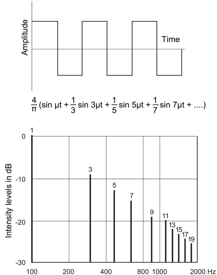
**Figure 10.** Spectral content of a perfect square wave
