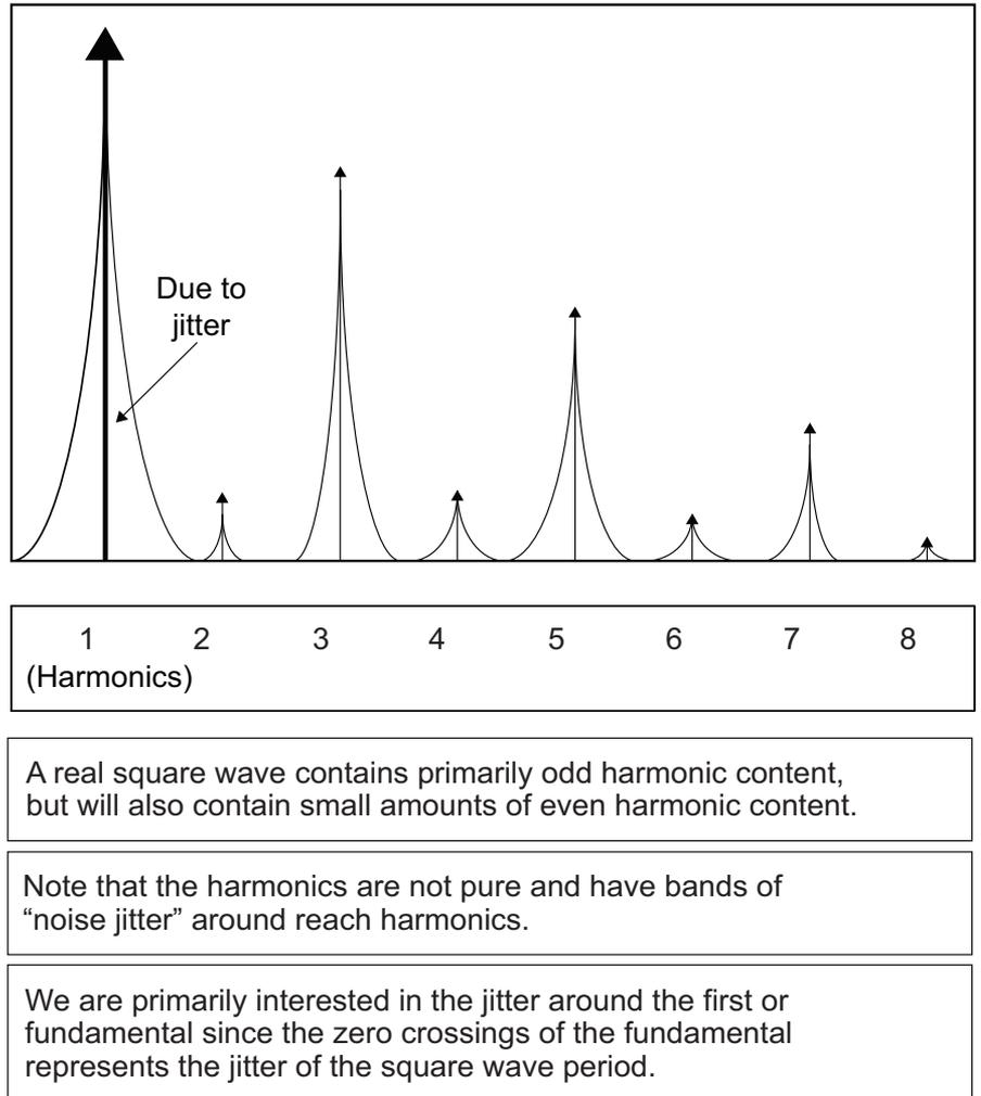
**Figure 11.** Spectral content of a realistic timing signal
