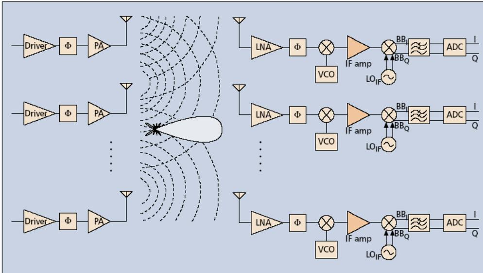
Figure 3: A generic multi-antenna transceiver architecture employing beam steering
