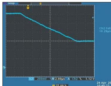
**Figure 5.  $V_{OUT}$  Max to Min Settling Time with No Load**
