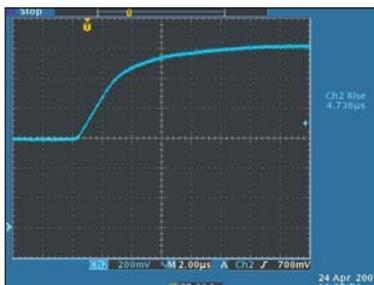
**Figure 4.  $V_{OUT}$  Min to Max Settling Time with No Load**
