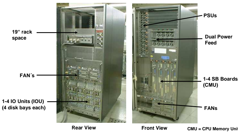
Figure 2-7. Fujitsu Siemens Computers SPARC Enterprise M8000 server enclosure diagram.
