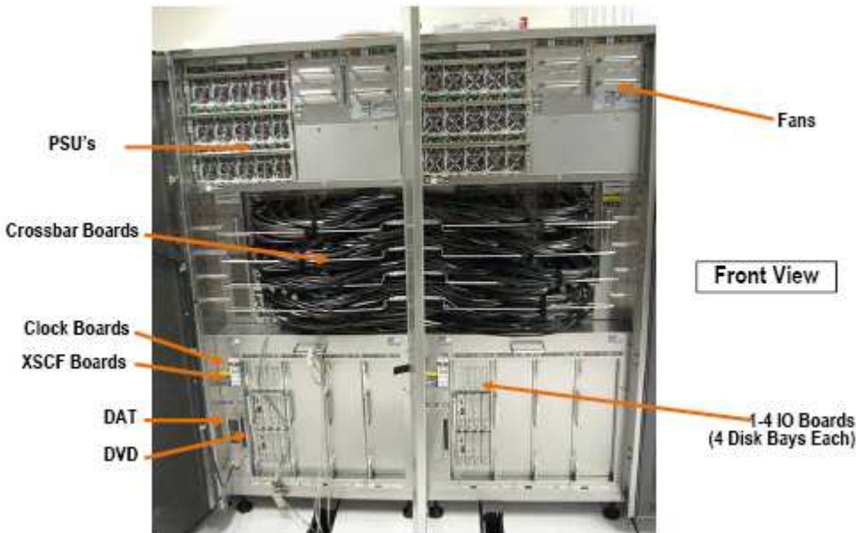
Figure 2-9. Fujitsu Siemens Computers SPARC Enterprise M9000-64 server enclosure diagram.
